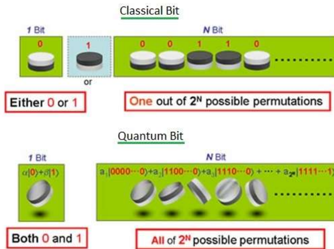
Figure 2: Classical bit vs. Quantum bit courtesy of www.rfwireless-world.com
